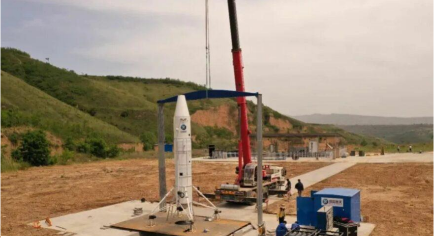
Preparations for a static fire test of the Nebula-M test stage in July 2021. Credit: Deep Blue Aerospace
