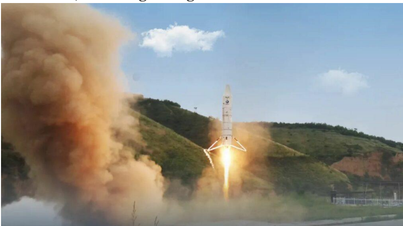
A hop test of Deep Blue Aerospace's Nebula-M test stage in July 2021. Credit: Deep Blue Aerospace
